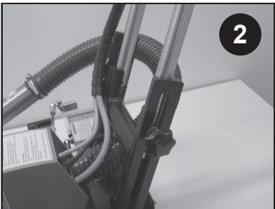
2. Fold up the handle and adjust to suitable height for the operator.
