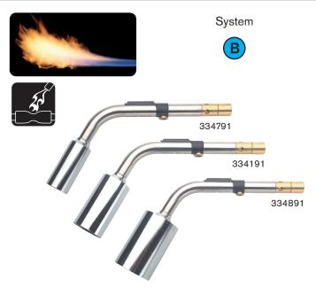
• Soft flame design ideal for cable work and other heat shrinking applications • Soft flame burners with sweeping, powerful yellow and blue soot-free windproof flames • Fresh air sucks in and keeps the burner head cold to minimize the risk of burning the shrink material • To heat the sleeves efficiently but still soft enough not to overheat the shrink material • Working pressure 2 bar
