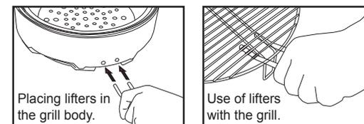
Placing lifters in the grill body.
